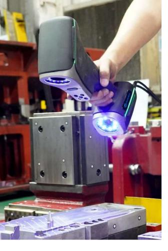
The **KSCAN-Magic** upgrade series is an advanced 3D scanner with infrared and blue lasers, five operating modes, and efficient multi-spectrum scanning. It optimizes workflows with fast scanning, high accuracy, and accelerates product time-to-market.
